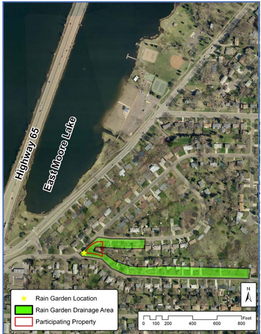
Curb-cut rain garden location and corresponding drainage area.
